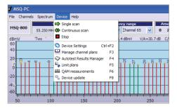
With the MSQ-900 connected to the MSQ-PC, users can access meter settings, channel plans, limit plans, and Autotest results.
