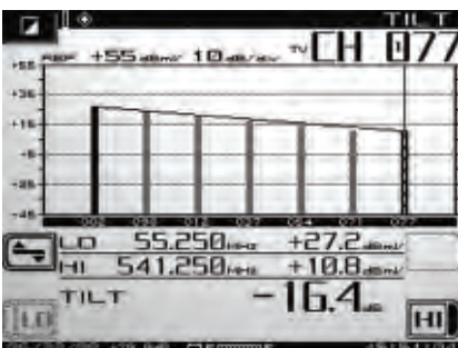
Tilt mode performs automatic tilt calculations between any two of nine designated carriers
